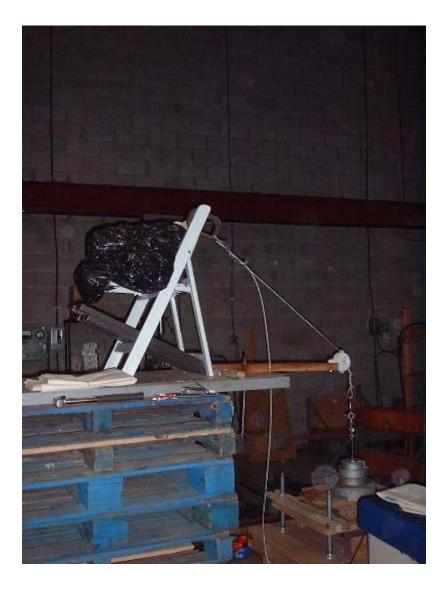
FIGURE 1 Back Durability Test Set-up
