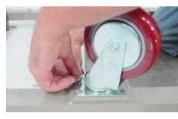
Install the wheels. **2** There is a short and long bolt. Install the short bolts on the inner side of the cart. Insert the bolt from the top, down towards the wheel. Put flat washer on then nut. tighten with allan key and wrench.
