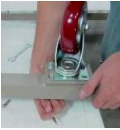
Repeat step 1 with long bolt on outer side of cart.
