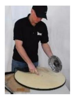
Center the coupler on the table using the center punch mark.
