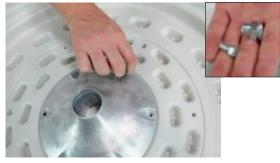
Insert steel plug and thread the bolt through the coupler and table top into the plug. Repeat for all 3 metal plugs.
