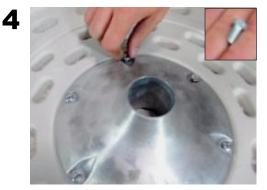
Screw in 3 bolts into remaining three holes.
