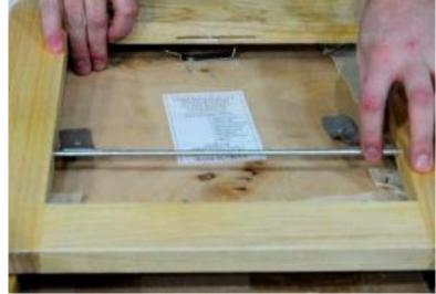
With one hand continuing to push the seat pad down, gently slide out the hook off the metal bar.
