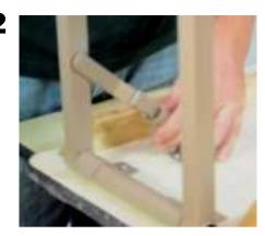
Slide the ring above the joint to lock in place
