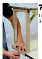
Tighten butterfly nut on Both sides
