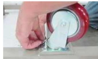
Install the wheels. **2**There is a short and long bolt. Install the short bolts on the inner side of the cart. Insert the bolt from the top, down towards the wheel. Put the washer on, then the nut. Tighten with allan key and wrench.
